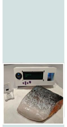
FIGURE 5 A prototype Conservation X labs DNA scanner. These portable scanners could be used to identify seafood to species level and help to reduce seafood fraud. Credit: Conservation X
