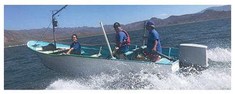
**FIGURE 1** A FlyWire camera system mounted on a small fishing vessel in the Gulf of California, Mexico. Source: FlyWire.com
