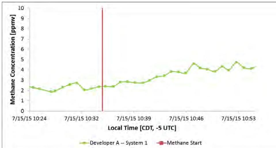
Figure A.2. Developer A Data Trace for a 1-scfm Leak from 50 ft of Distance
