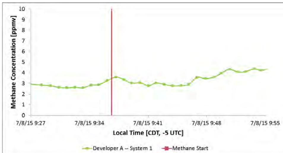
Figure A.14. Developer A Data Trace for a 5-scfm Leak from 82 ft of Distance
