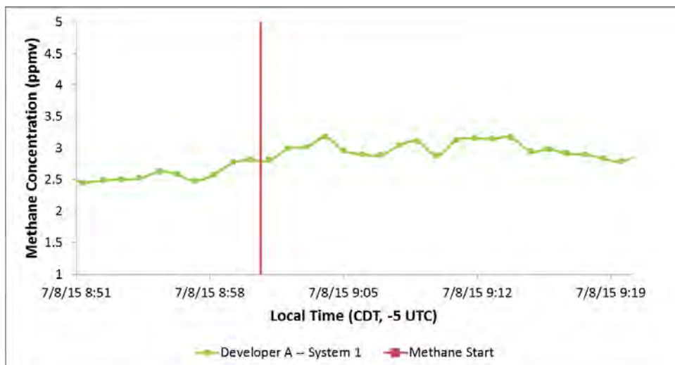
Figure A.9. Developer A Data Trace for a 2.5-scfm Leak from 82 ft of Distance
