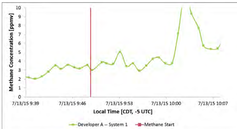
Figure A.6. Developer A Data Trace for a 2.5-scfm Leak from 30 ft of Distance
