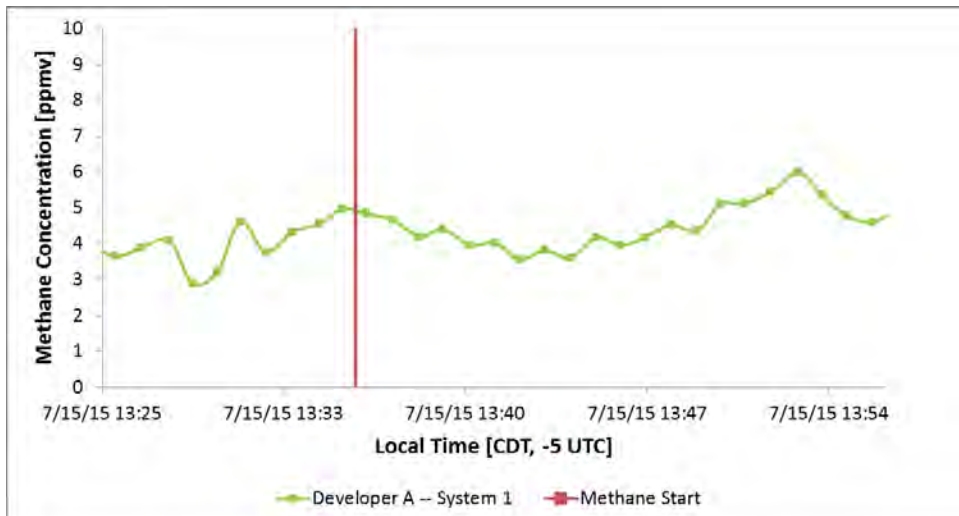
Figure A.3. Developer A Data Trace for a 1-scfm Leak from 70 ft of Distance
