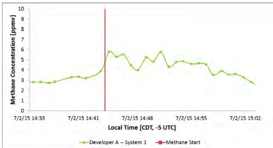
Figure A.12. Developer A Data Trace for a 5-scfm Leak from 50 ft of Distance
