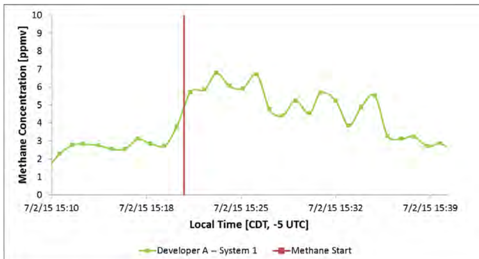
Figure A.11. Developer A Data Trace for a 5-scfm Leak from 30 ft of Distance
