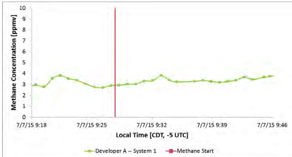
Figure A.7. Developer A Data Trace for a 2.5-scfm Leak from 50 ft of Distance
