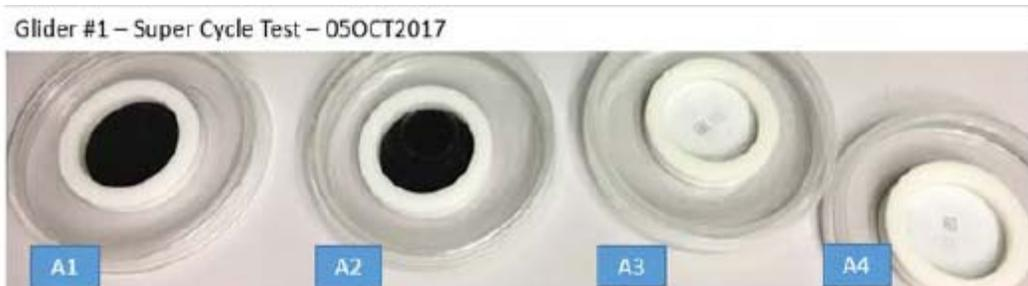
**Figure 9: PM Filters from Glider #1 testing over the Super Cycle Test<sup>2</sup>**
