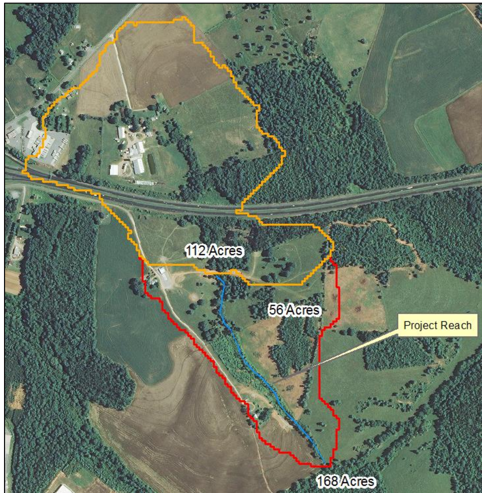
Figure 9: Catchment Delineation Example for Reach Runoff.
