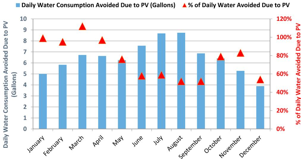
Fig. 11. Daily grid-related water consumption avoided due to a 5.61 KW PV array in absolute and percentage terms, by month.
