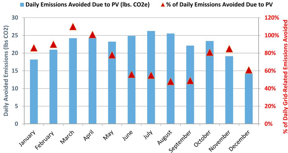
Fig. 10. Daily CO<sub>2</sub> grid emissions avoided due to a 5.61 KW PV array in absolute and percentage terms, by month.
