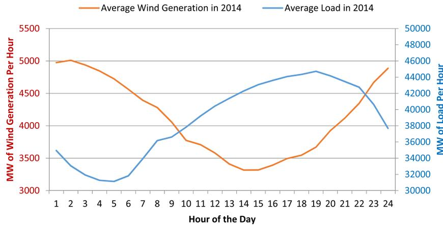
Fig. 2. Average wind generation and load in 2014 in ERCOT region.<sup>a</sup> Data Source: <http://www.ercot.com/gridinfo/generation/>
