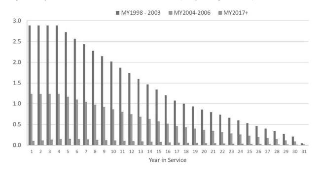
Figure 3 Projected Annual PM Emissions, Class 8 Tractors (tons/year/original vehicle)
