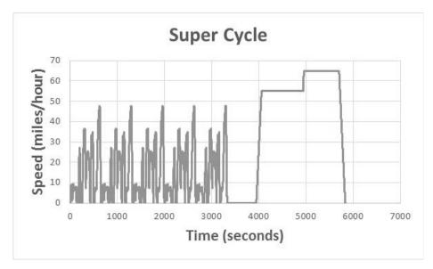
Figure 3: Super Cycle speed vs. time profile
