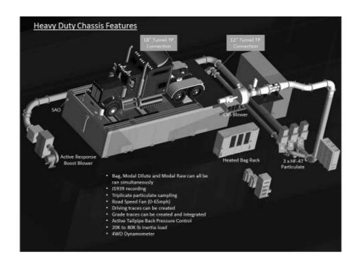
Figure 8: Chassis Dynamometer Overview
