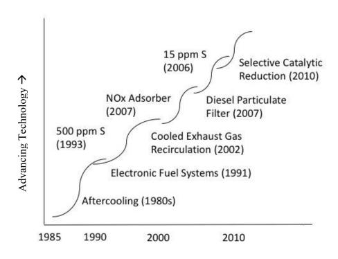
Fig. 1. Evolution of diesel emission control technology in the U.S. Source: John Wall.
