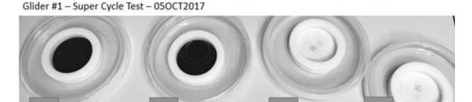
Figure 9: PM Filters from Glider #1 testing over the Super Cycle Test<sup>2</sup>
