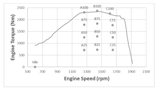
Figure 4: Glider #2 torque curve and SET test points
