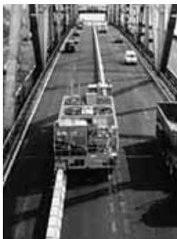
This machine is shifting a moveable lane barrier to add an extra lane in the congested direction.
