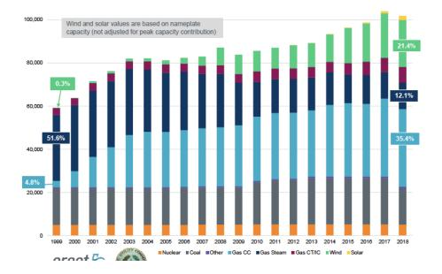
Figure 3 -- ERCOT Installed Capacity, 1999 through 2018<sup>17</sup>
