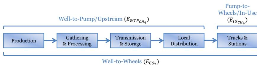
**Figure 1.** Natural gas value chain schematic. The aggregations of the value chain in this paper include estimates for all CH<sub>4</sub> and CO<sub>2</sub> emissions (fugitive, vented, and combustion) from all equipment in each industry segment (Supporting Information, section S4).
