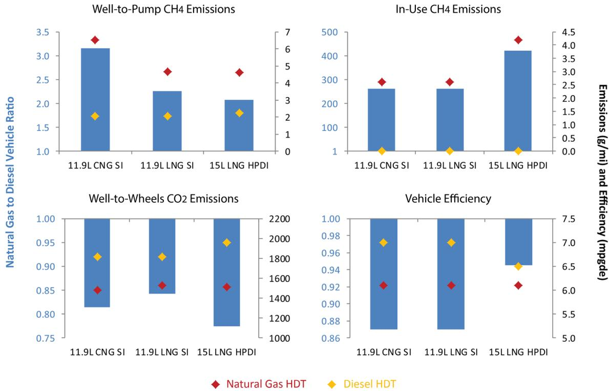
**Figure 2.** Reference case assumptions for all three natural gas fuel switching scenarios. Assumptions are expressed as absolute values (yellow and red points, right axis) and as the ratio of natural gas over diesel HDT values (bars, left axis).
