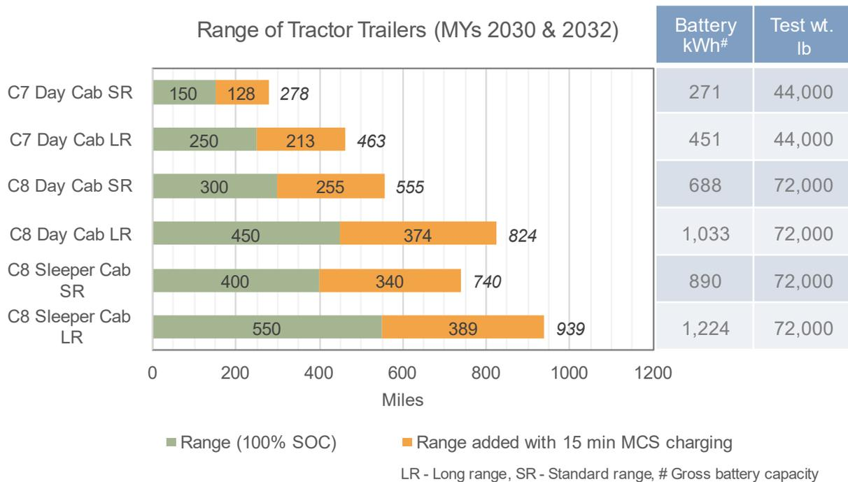
**Figure 1: Battery size (kWh), range (miles), test weight (lb), and the range added with a 15-minute charging session at a Megawatt Charging System (MCS) station.**
