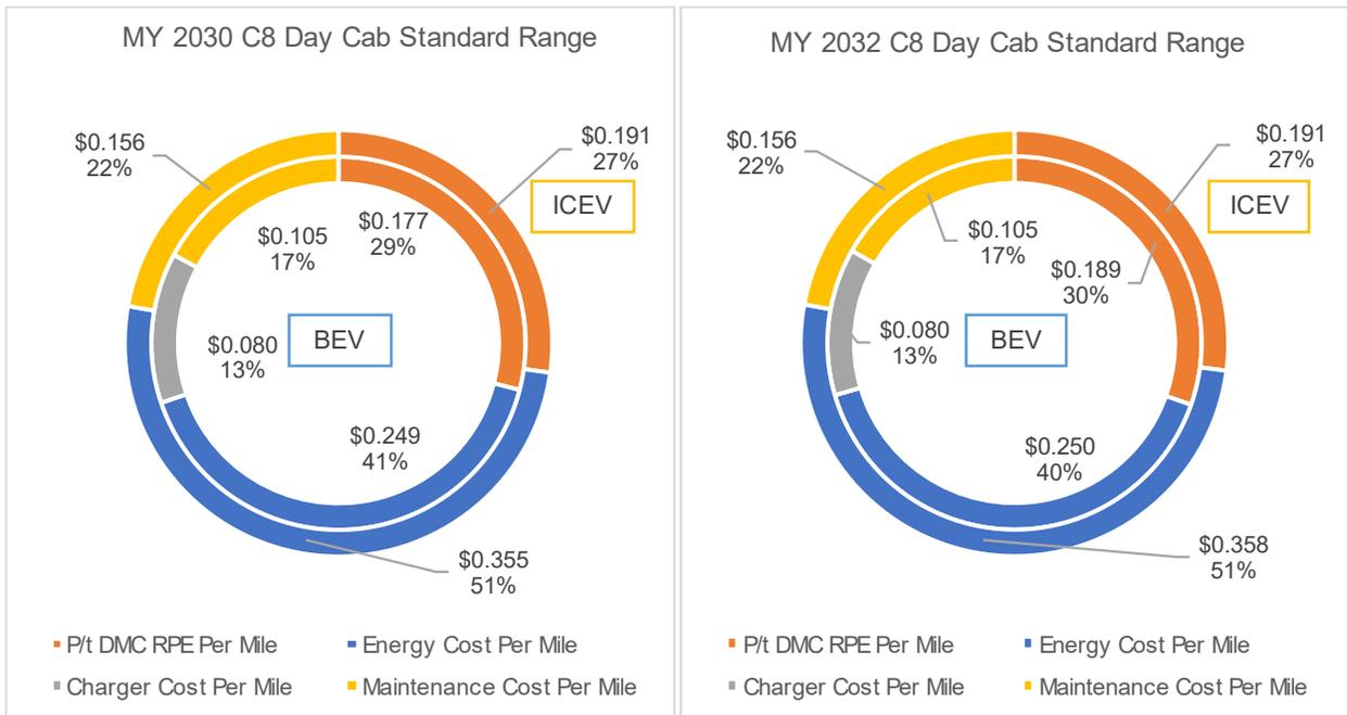
**Figure 73: MYs 2030 and 2032 Class 8 Day Cab Standard Range ICEV and BEV contributions to TCO in a mixed charging scenario**
