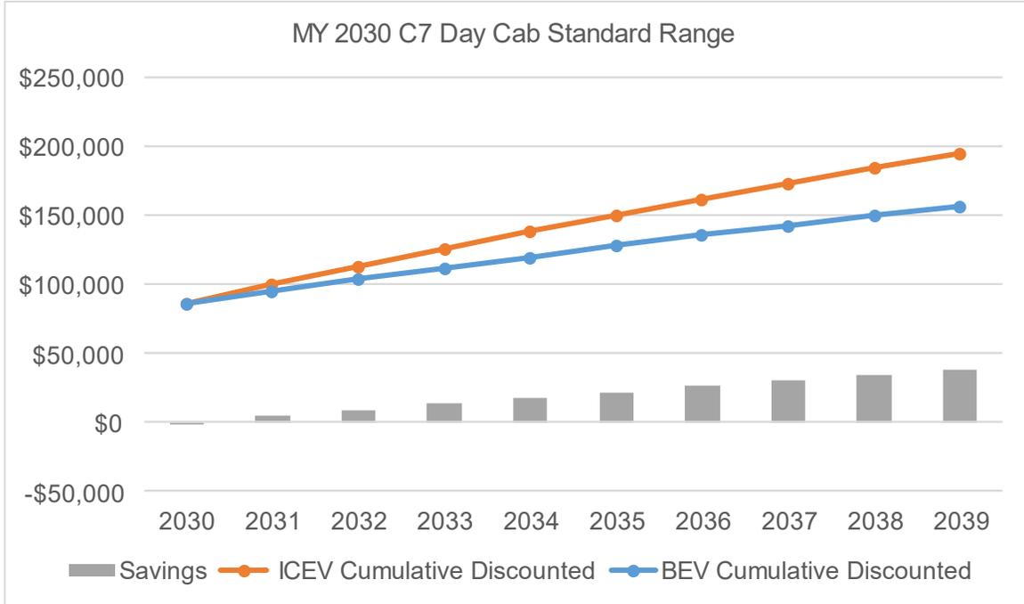
**Figure 68: TCO parity of an MY 2030 Class 7 day cab standard range with mixed charging scenario.**
