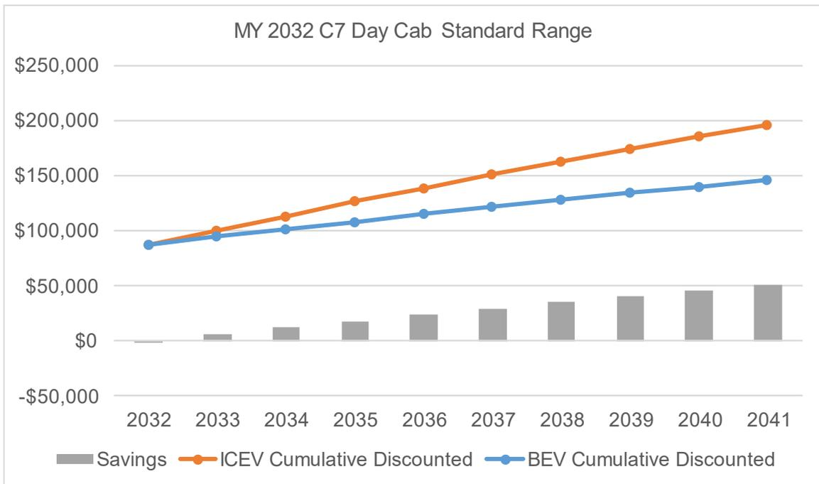
**Figure 57: TCO parity of an MY 2032 Class 7 day cab standard range with depot charging.**
