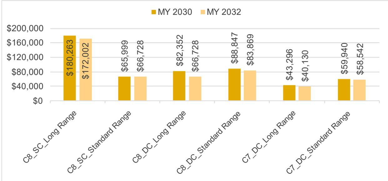
**Figure 77: Cumulative Net Savings of BEVs over ICEVs in MYs 2030 and 2032 without discounting**
