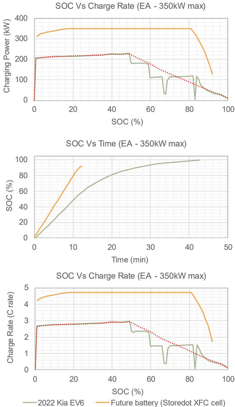
**Figure 23: Charging a 2022 Kia EV6 [53], and an equivalent StoreDot XFC cell-based battery pack [54] (calculated based on cell performance) on an EA 350kW charger**
