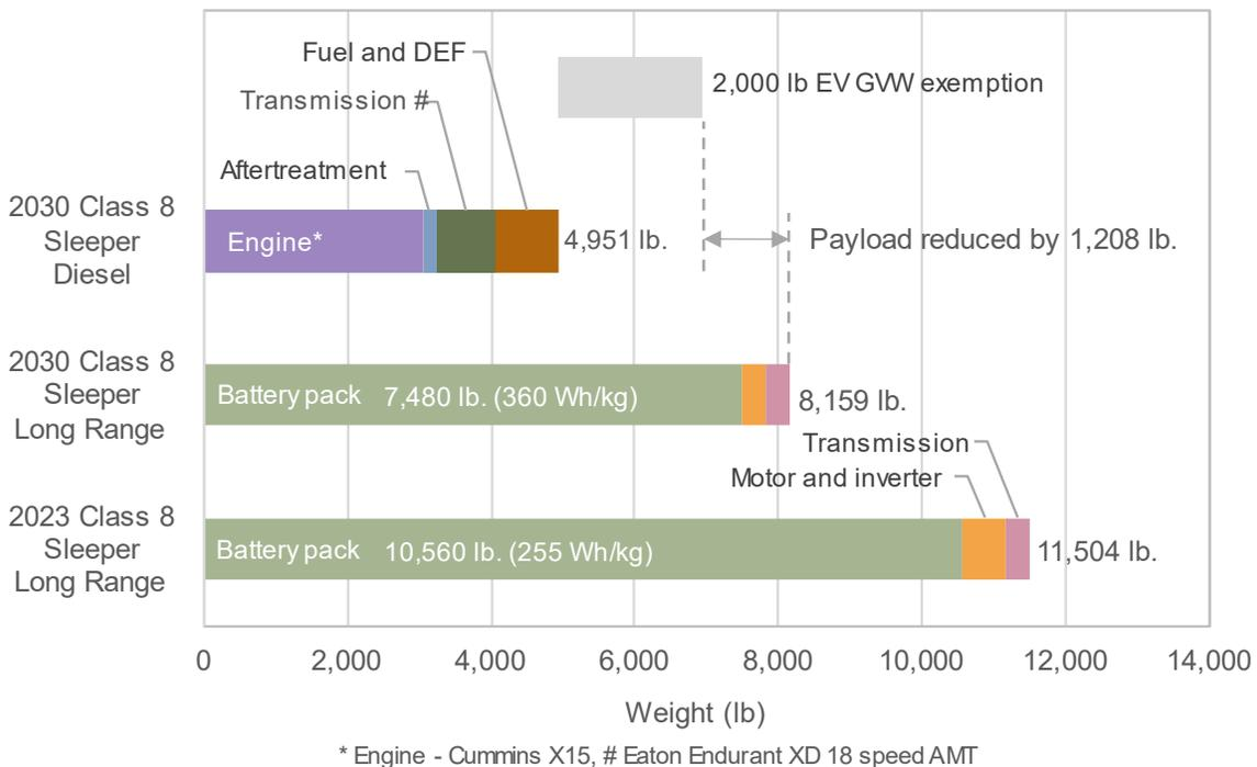
**Figure 2: Comparison of the powertrain weight of Class 8 Sleeper long-range diesel and electric powertrains, respectively**
