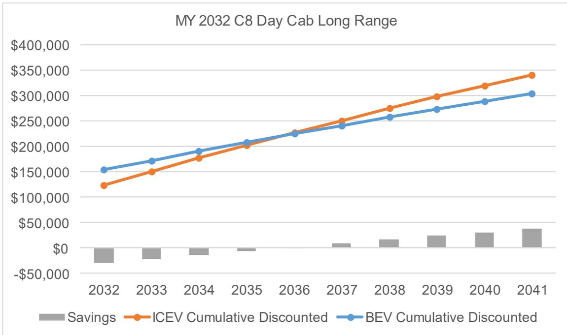
**Figure 63: TCO parity of an MY 2032 Class 8 day cab long range with mixed charging scenario.**
