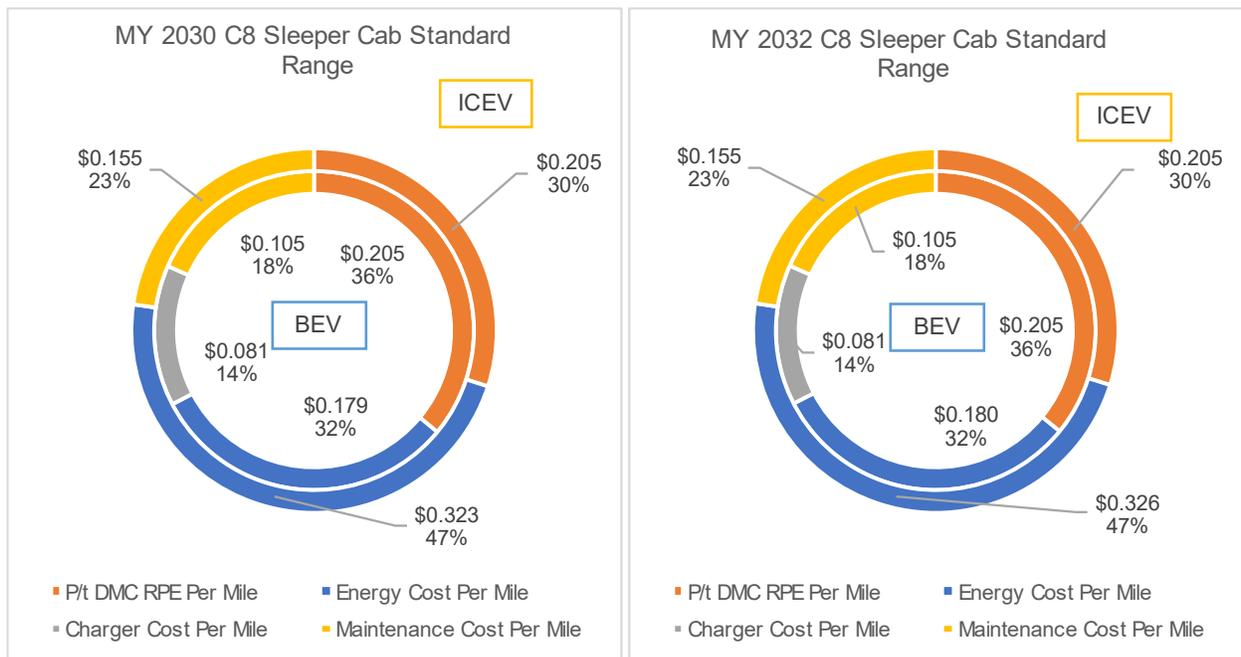
**Figure 30: MYs 2030 and 2032 Class 8 Sleeper Cab Standard Range ICEV and BEV contributions to TCO. P/t stands for Powertrain.**
