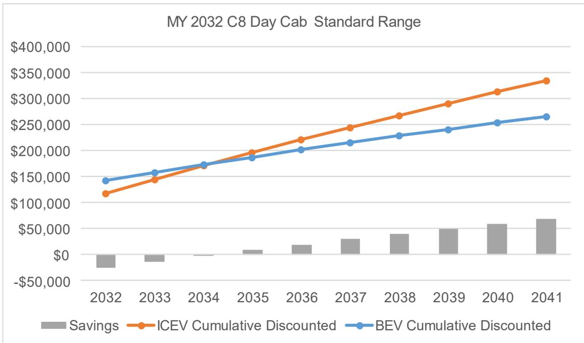
**Figure 53: TCO parity of an MY 2032 Class 8 day cab standard range with depot charging.**
