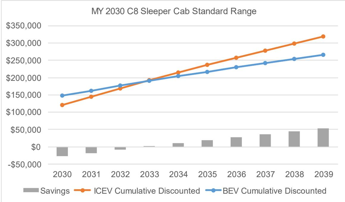
**Figure 48: TCO parity of an MY 2030 Class 8 sleeper cab standard range with depot charging.**
