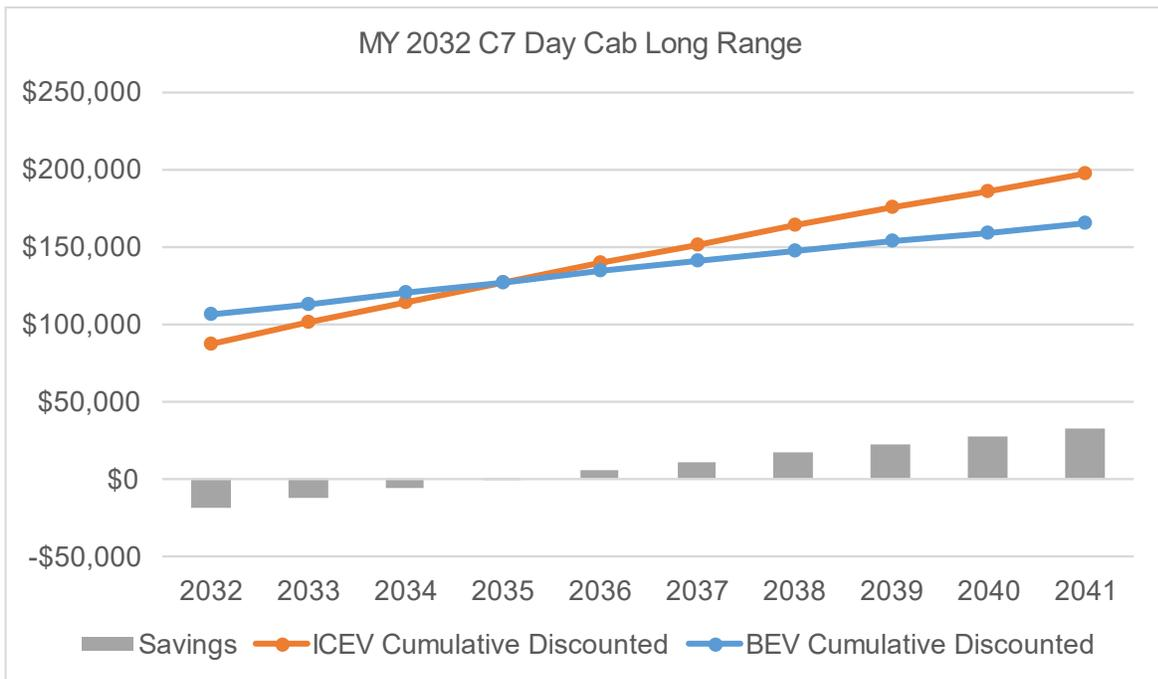
**Figure 55: TCO parity of an MY 2032 Class 7 day cab long range with depot charging.**
