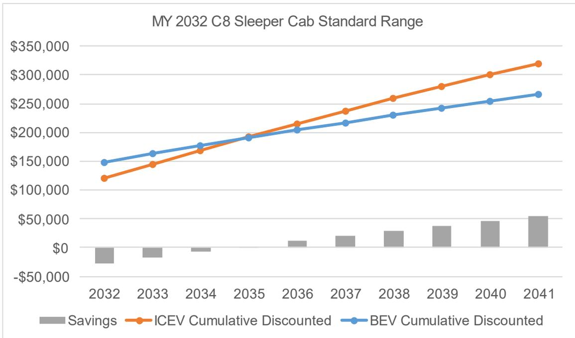
**Figure 49: TCO parity of an MY 2032 Class 8 sleeper cab standard range with depot charging.**
