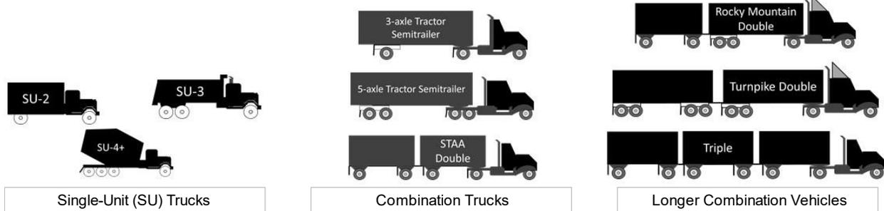
**Figure 10: Common Vehicle Configurations in the U.S. Commercial Truck Fleet [7]**
