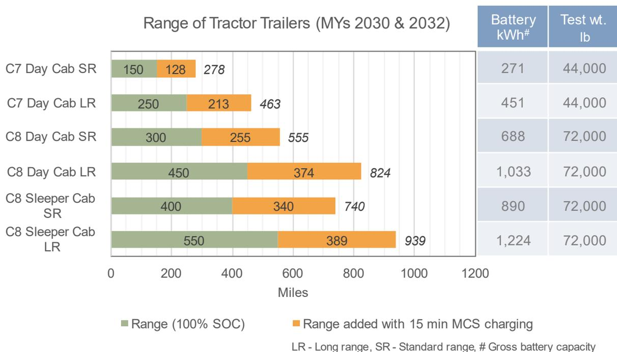
**Figure 25: Battery size (kWh), range (miles), Test weight (lb), and the range added with a 15-minute charging session at a 3,000 Amp Megawatt Charging System (MCS) station**
