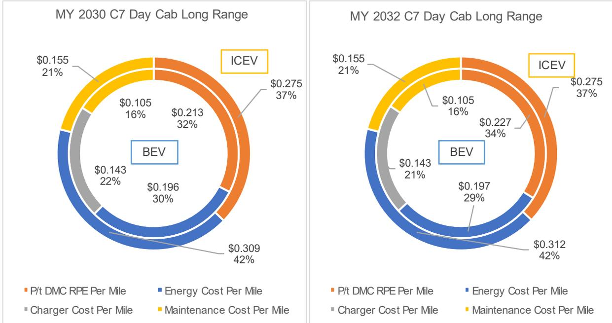
**Figure 74: MYs 2030 and 2032 Class 7 Day Cab Long Range ICEV and BEV contributions to TCO in a mixed charging scenario**
