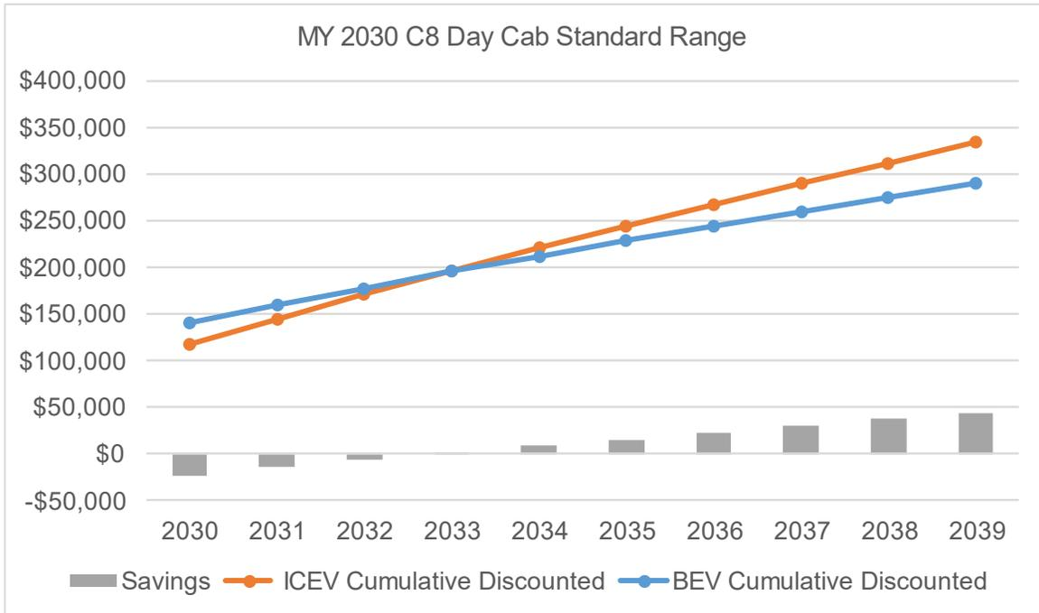
**Figure 64: TCO parity of an MY 2030 Class 8 day cab standard range with mixed charging scenario.**
