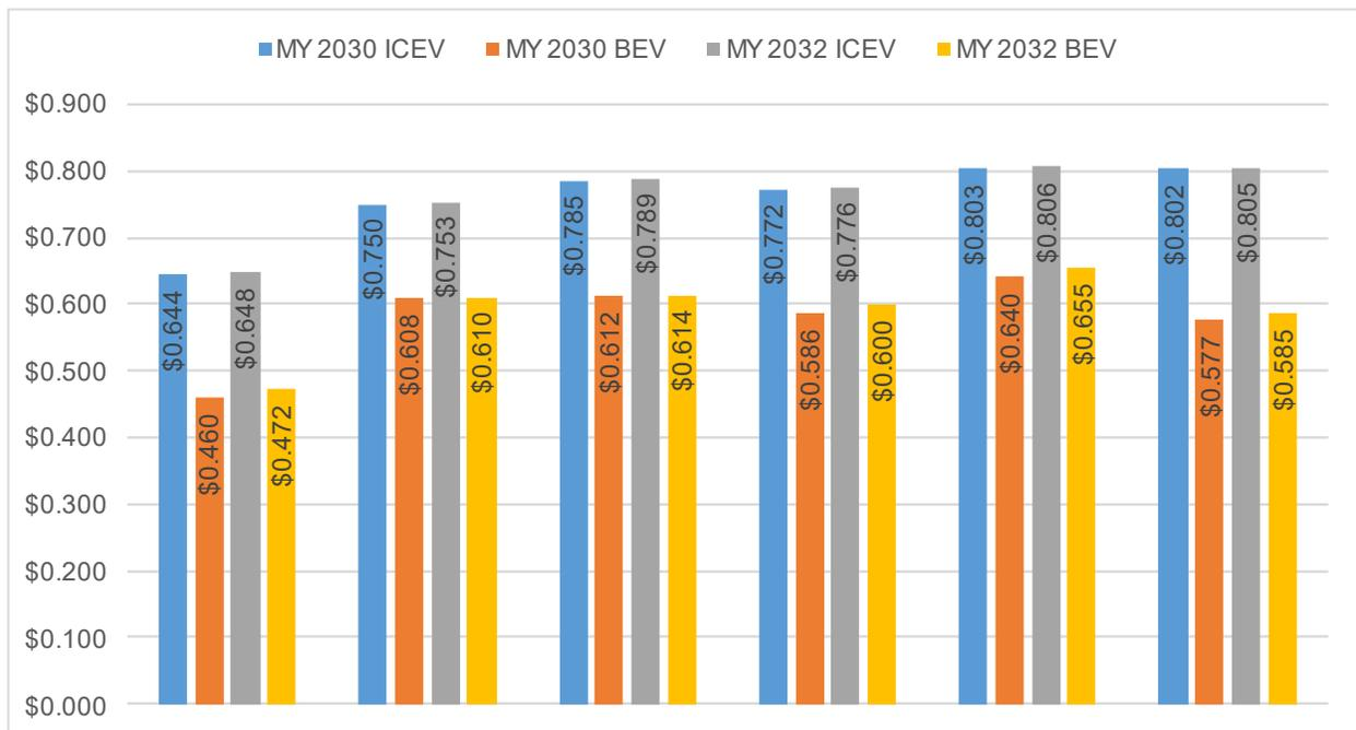
**Figure 76: TCO per mile of ICEVs and BEVs in MYs 2030 and 2032 without discounting**
