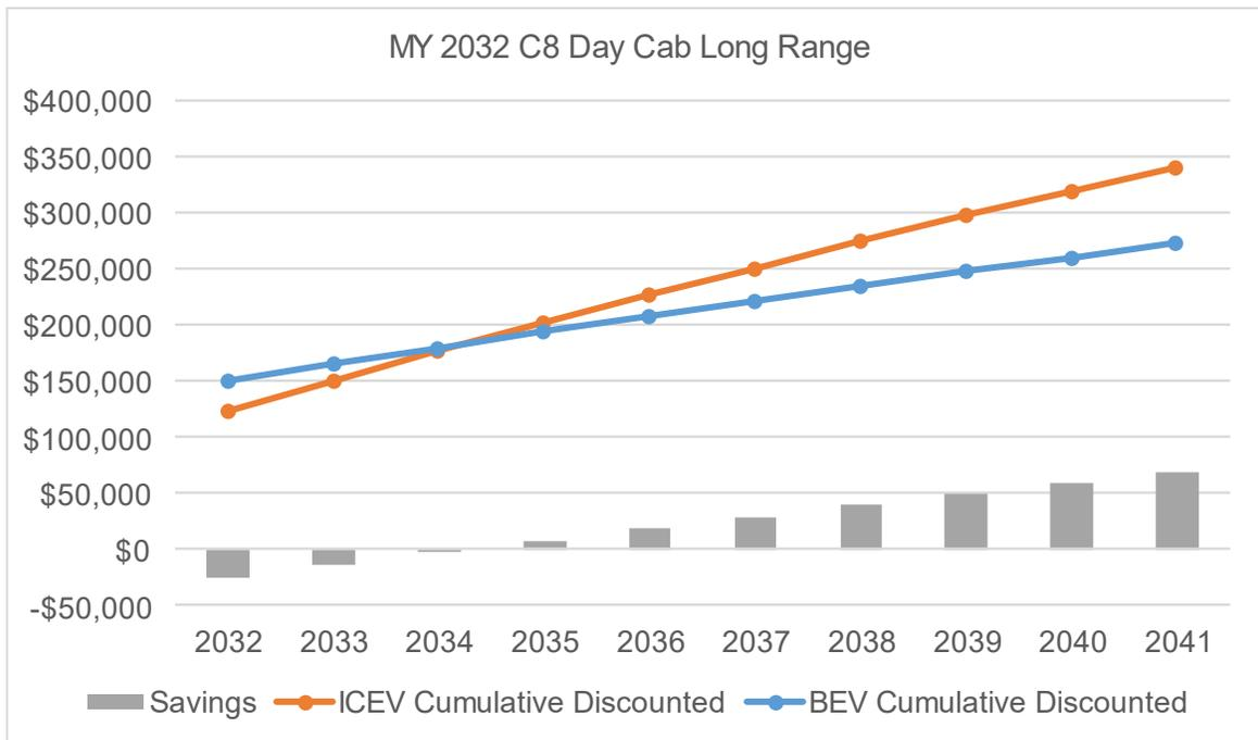
**Figure 51: TCO parity of an MY 2032 Class 8 day cab long range with depot charging.**
