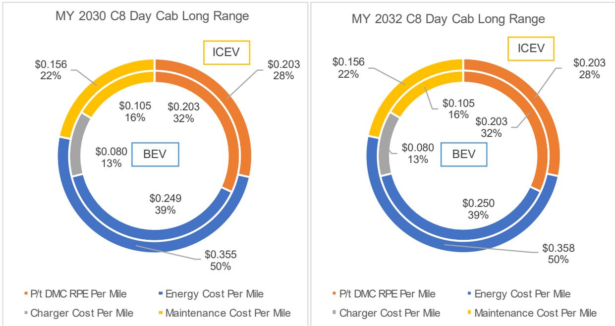
**Figure 72: MYs 2030 and 2032 Class 8 Day Cab Long Range ICEV and BEV contributions to TCO in a mixed charging scenario**
