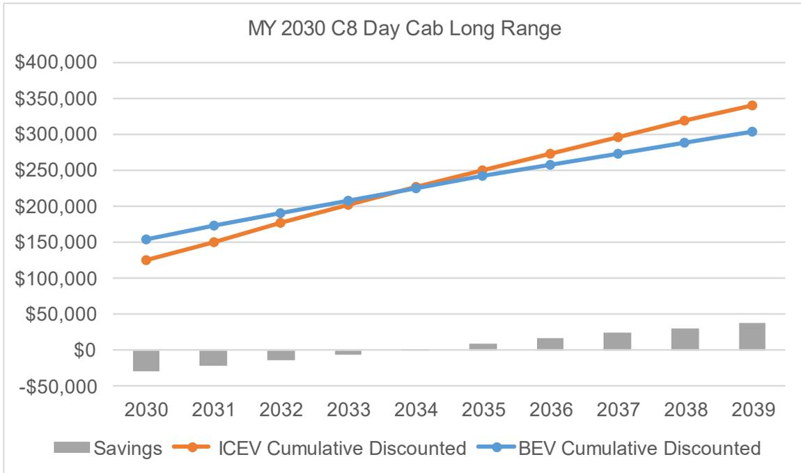
**Figure 62: TCO parity of an MY 2030 Class 8 day cab long range with mixed charging scenario.**
