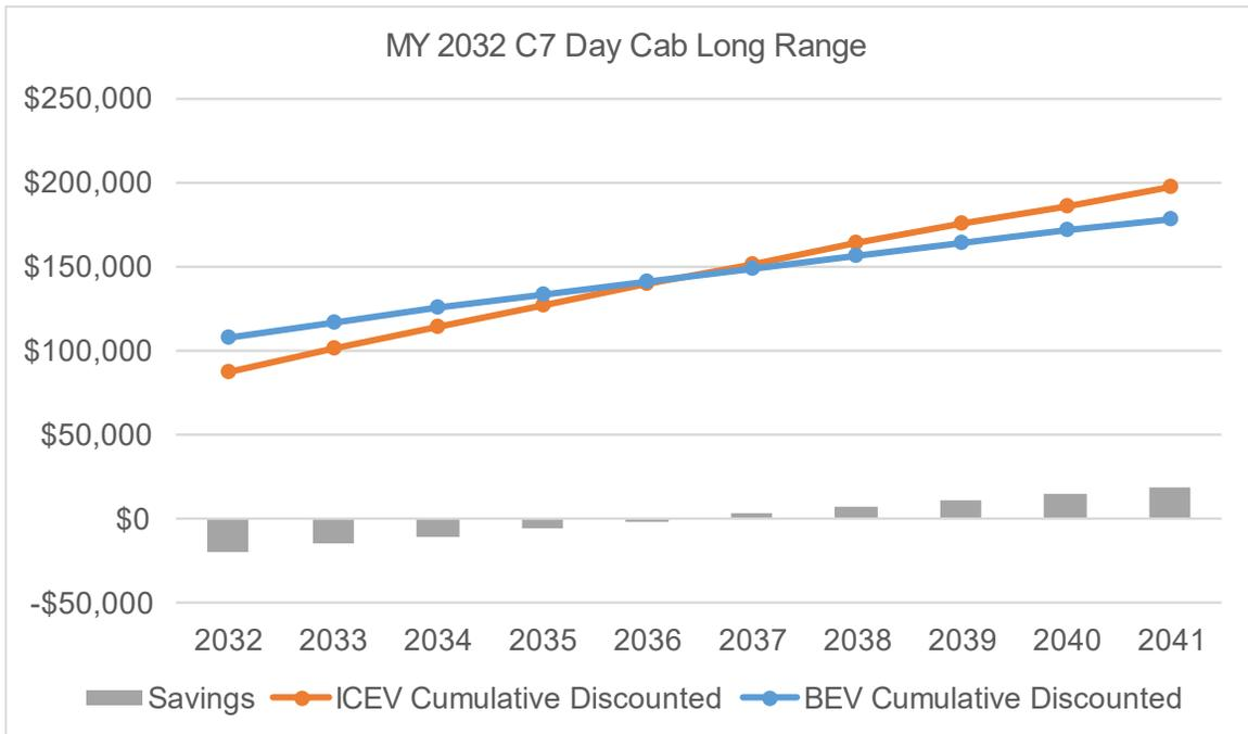
**Figure 67: TCO parity of an MY 2032 Class 7 day cab long range with mixed charging scenario.**
