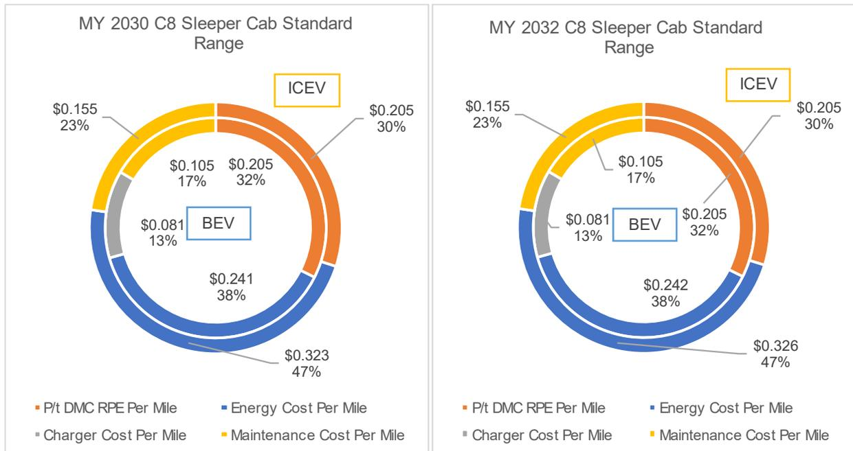
**Figure 71: MYs 2030 and 2032 Class 8 Sleeper Cab Standard Range ICEV and BEV contributions to TCO in a mixed charging scenario**
