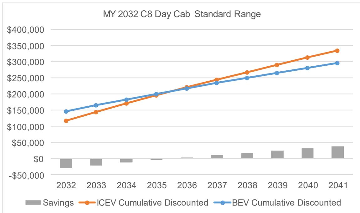
**Figure 65: TCO parity of an MY 2032 Class 8 day cab standard range with mixed charging scenario.**
