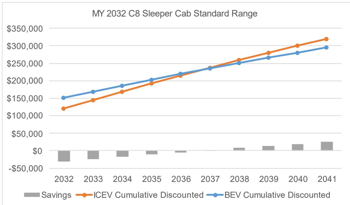
**Figure 61: TCO parity of an MY 2032 Class 8 sleeper cab standard range with mixed charging scenario.**
