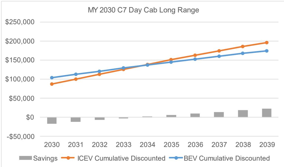
**Figure 66: TCO parity of an MY 2030 Class 7 day cab long range with mixed charging scenario.**
