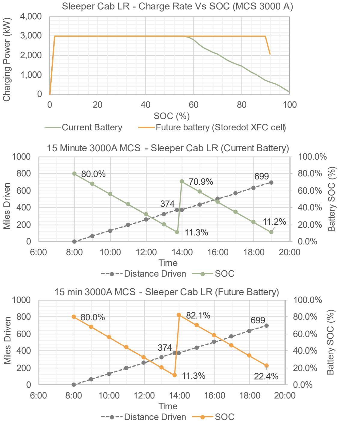
**Figure 24: (Top) Estimated peak charging rate for a Sleeper Cab LR (1224 kWh battery pack) with present and future battery technologies. (Middle and bottom) Driving a Sleeper Cab LR at 65 miles an hour, starting at 80% SOC. The vehicle is charged for 15 minutes at a 3000A MCS Dispenser starting at 11.3% SOC. The pack nominal voltage is 1000V.**
