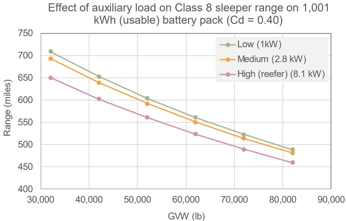
**Figure 22: Effect of auxiliary loads on energy efficiency**
