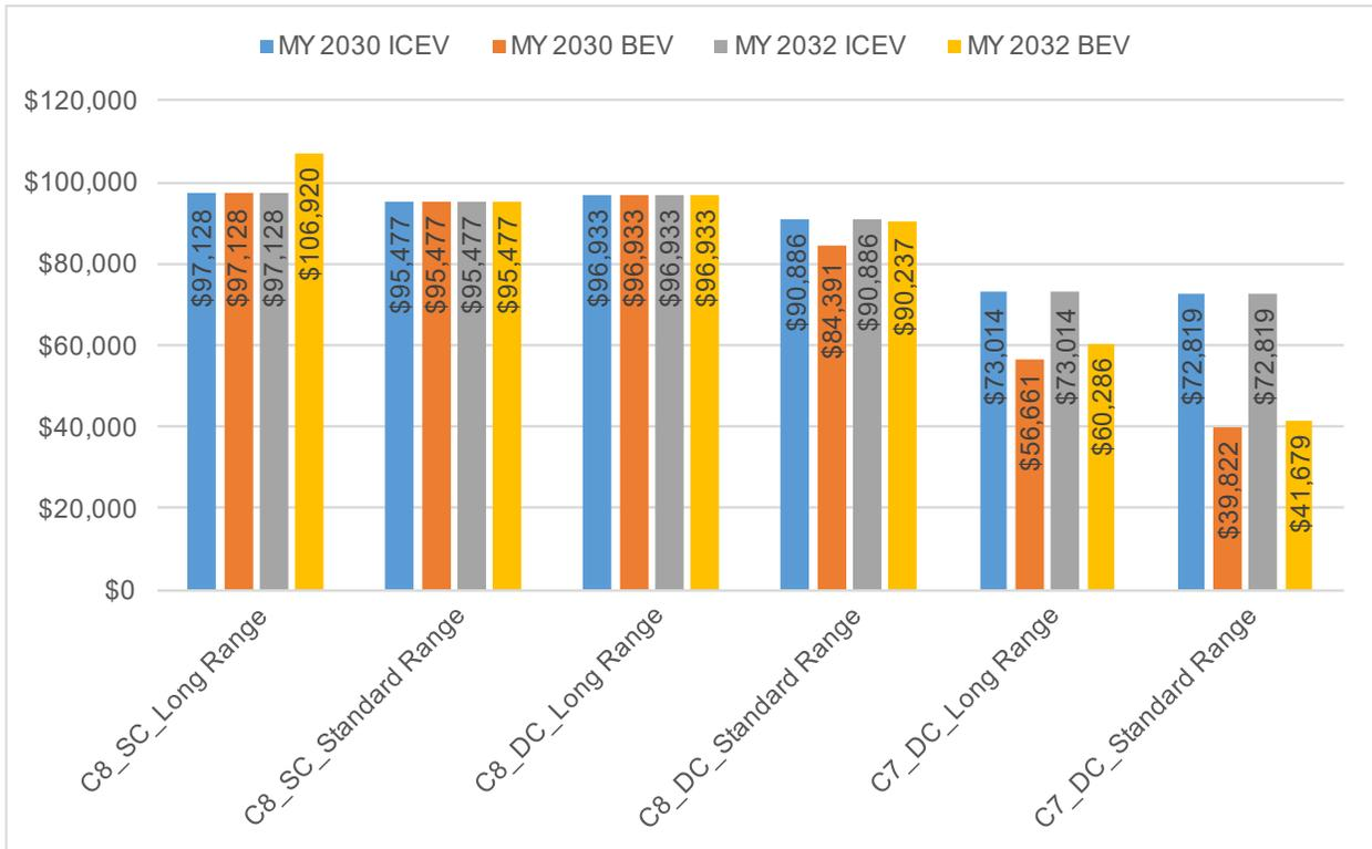
**Figure 27: Powertrain DMC with RPE of ICEVs and BEVs in MYs 2030 and 2032**
