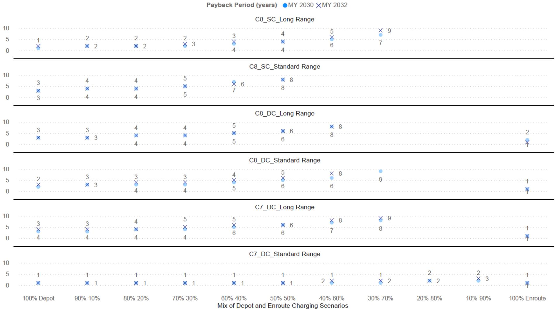
**Figure 41: Payback period of Class 7/8 trucks in a varying mix of the depot and en route charging scenarios. In scenarios with “End of life” cases, the respective markers are not shown.**
