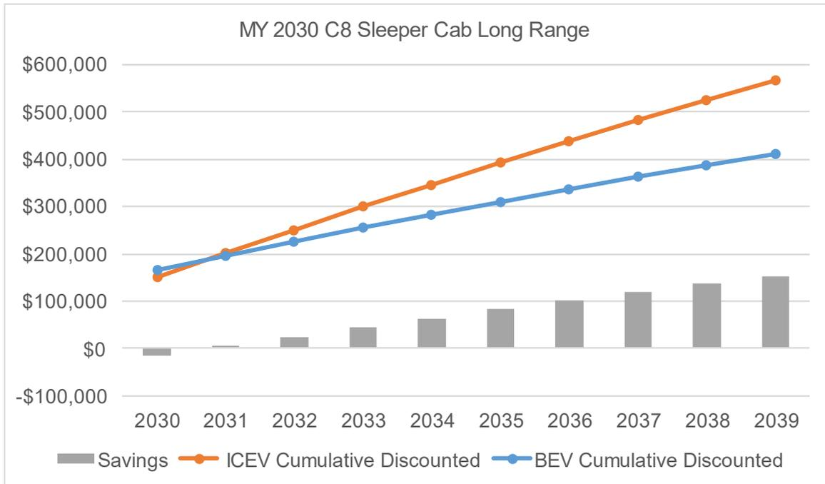
**Figure 46: TCO parity of an MY 2030 Class 8 sleeper cab long range with depot charging.**
