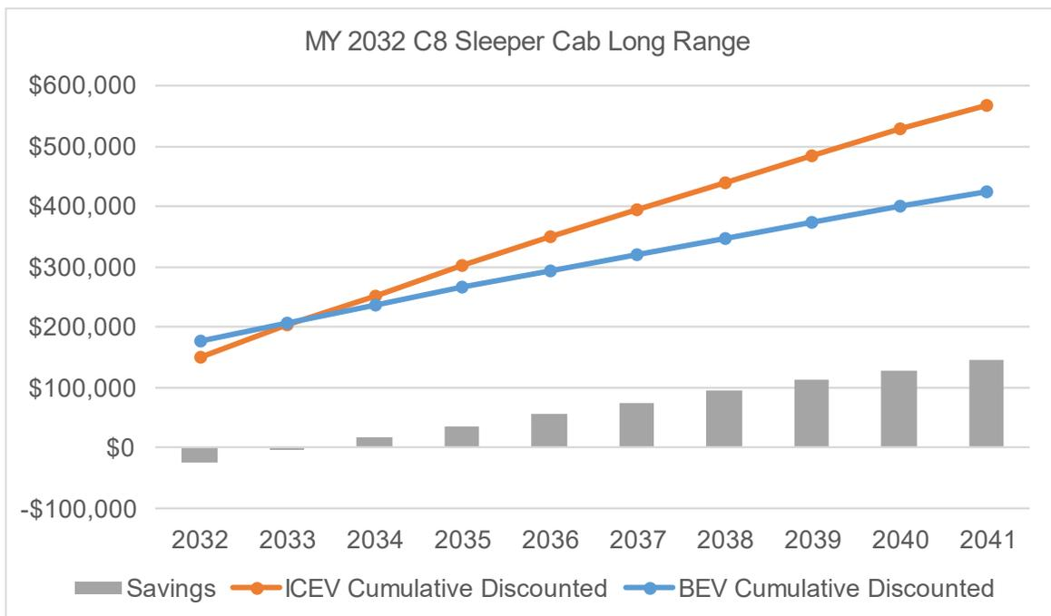
**Figure 47: TCO parity of an MY 2032 Class 8 sleeper cab long range with depot charging.**
