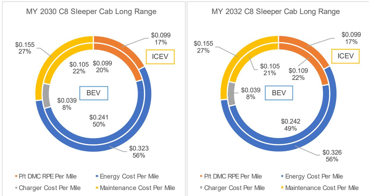
**Figure 70: MYs 2030 and 2032 Class 8 Sleeper Cab Long Range ICEV and BEV contributions to TCO in a mixed charging scenario**
