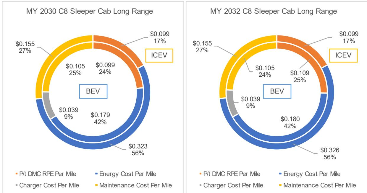
**Figure 29: MYs 2030 and 2032 Class 8 Sleeper Cab Long Range ICEV and BEV contributions to TCO. P/t stands for Powertrain.**
