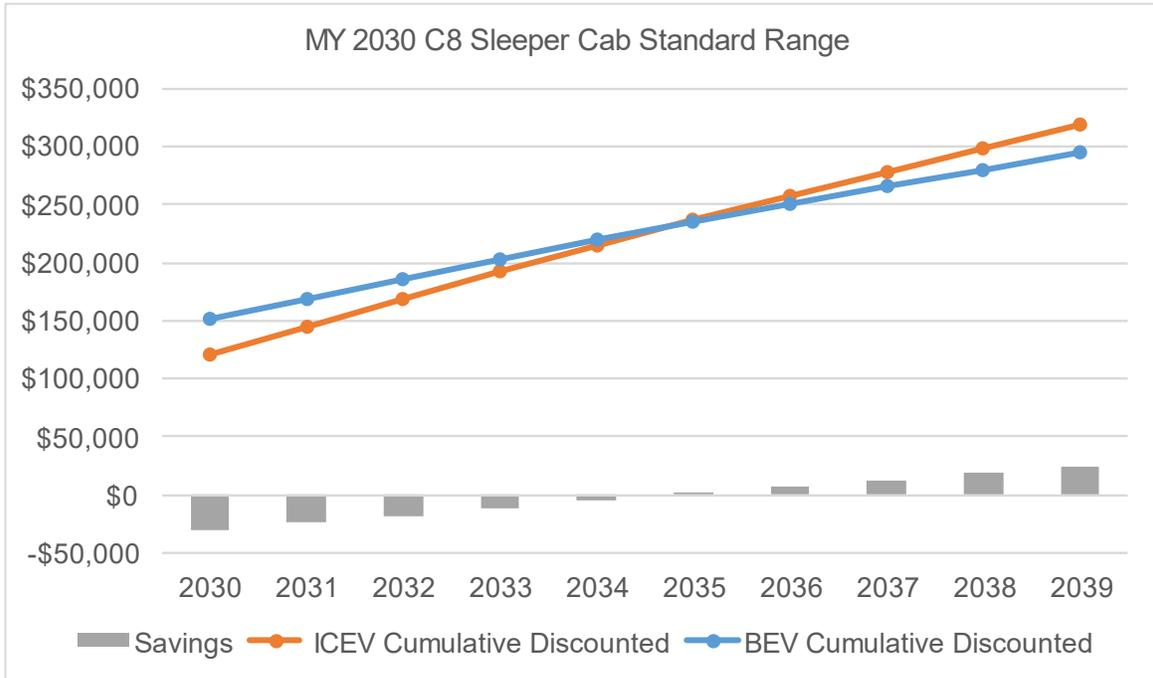
**Figure 60: TCO parity of an MY 2030 Class 8 sleeper cab standard range with mixed charging scenario.**
