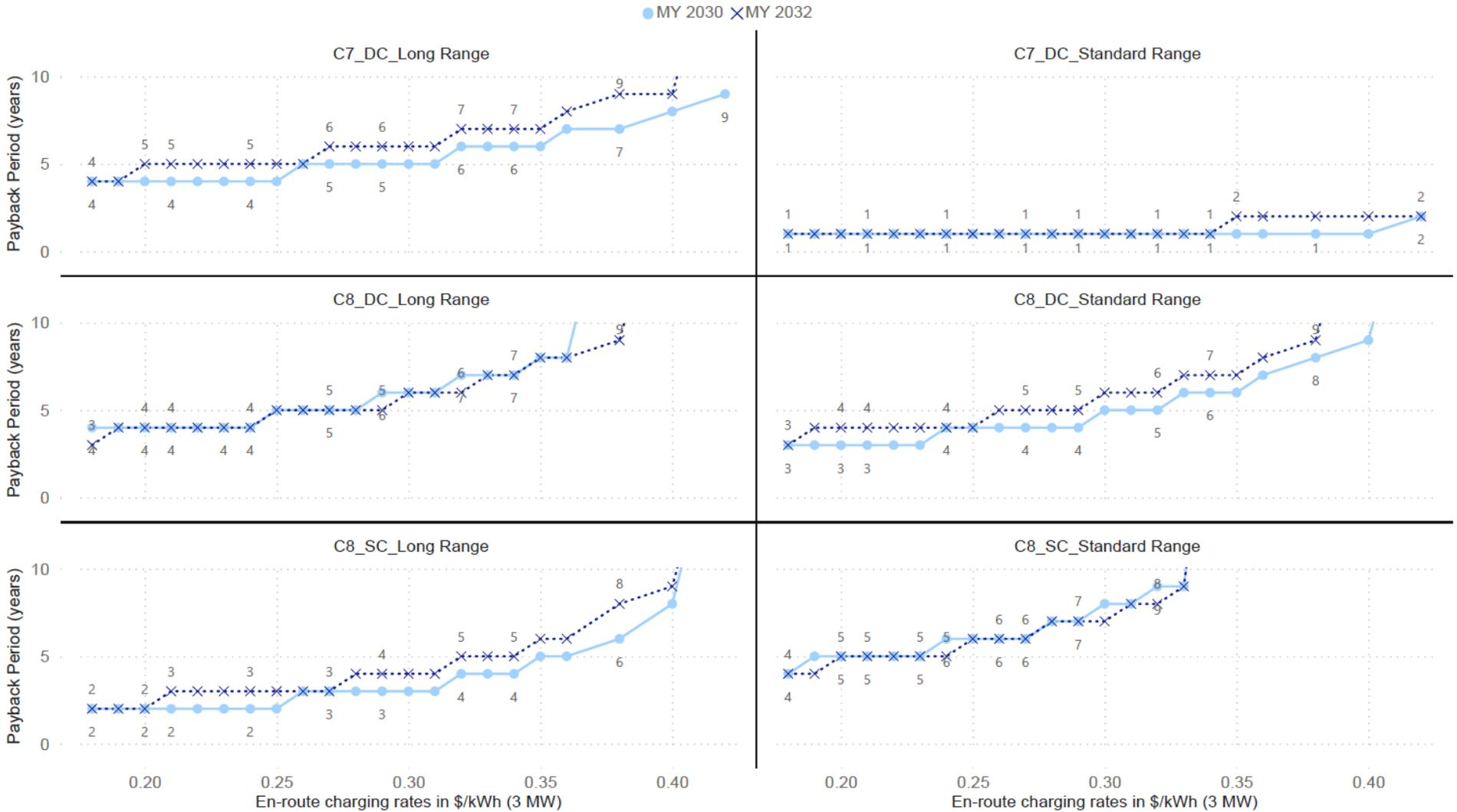
**Figure 42: Payback period of Class 7/8 trucks in a mixed charging scenario with varying charging rates in \$/kWh. In scenarios with “End of life” cases, the respective markers are not shown.**
