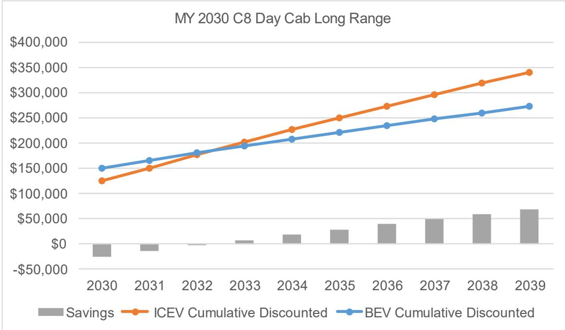
**Figure 50: TCO parity of an MY 2030 Class 8 day cab long range with depot charging.**
