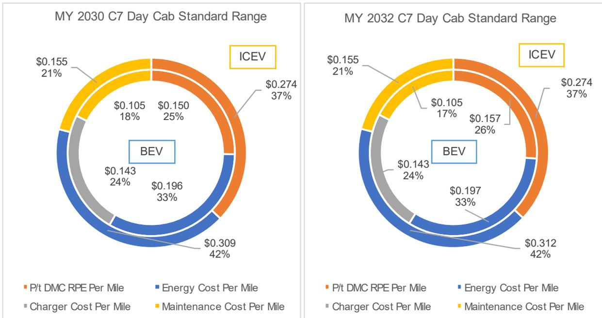
**Figure 75: MYs 2030 and 2032 Class 7 Day Cab Standard Range ICEV and BEV contributions to TCO in a mixed charging scenario**
