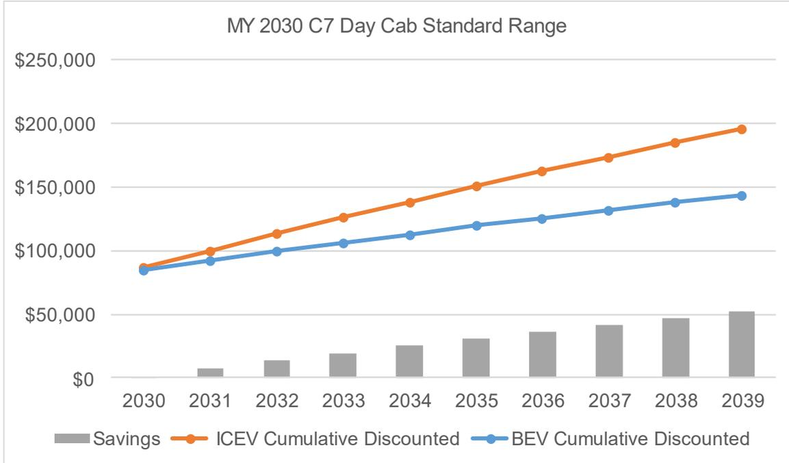
**Figure 56: TCO parity of an MY 2030 Class 7 day cab standard range with depot charging.**
