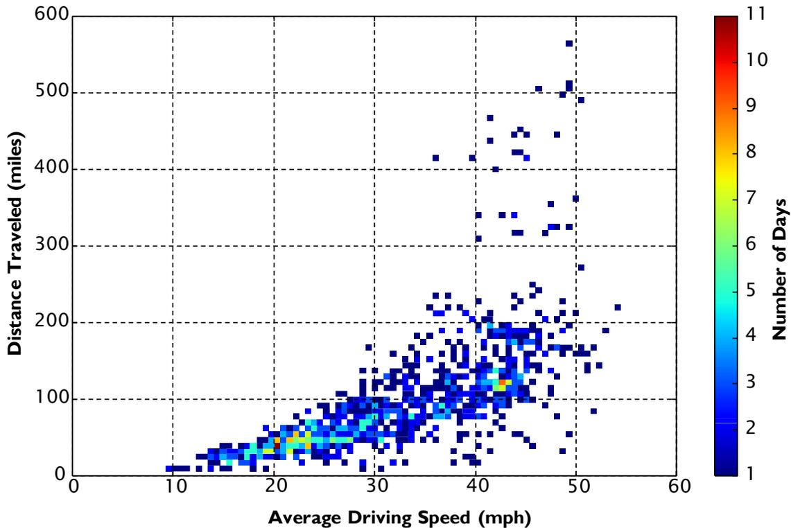
**Figure 16: Daily average driving speed vs. distance traveled for Class 8 traveled for Class 8. NREL Fleet DNA, 2014 [21]**
