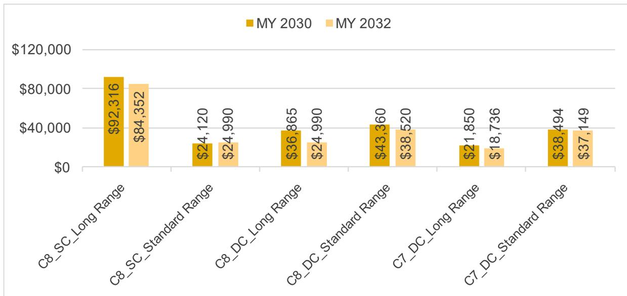
**Figure 40: Cumulative Net Savings of BEVs over ICEVs in a mixed charging scenario**
