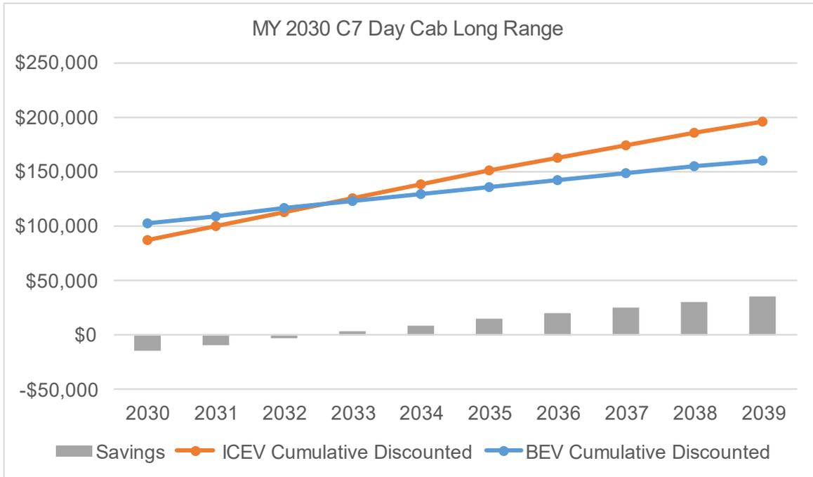
**Figure 54: TCO parity of an MY 2030 Class 7 day cab long range with depot charging.**
