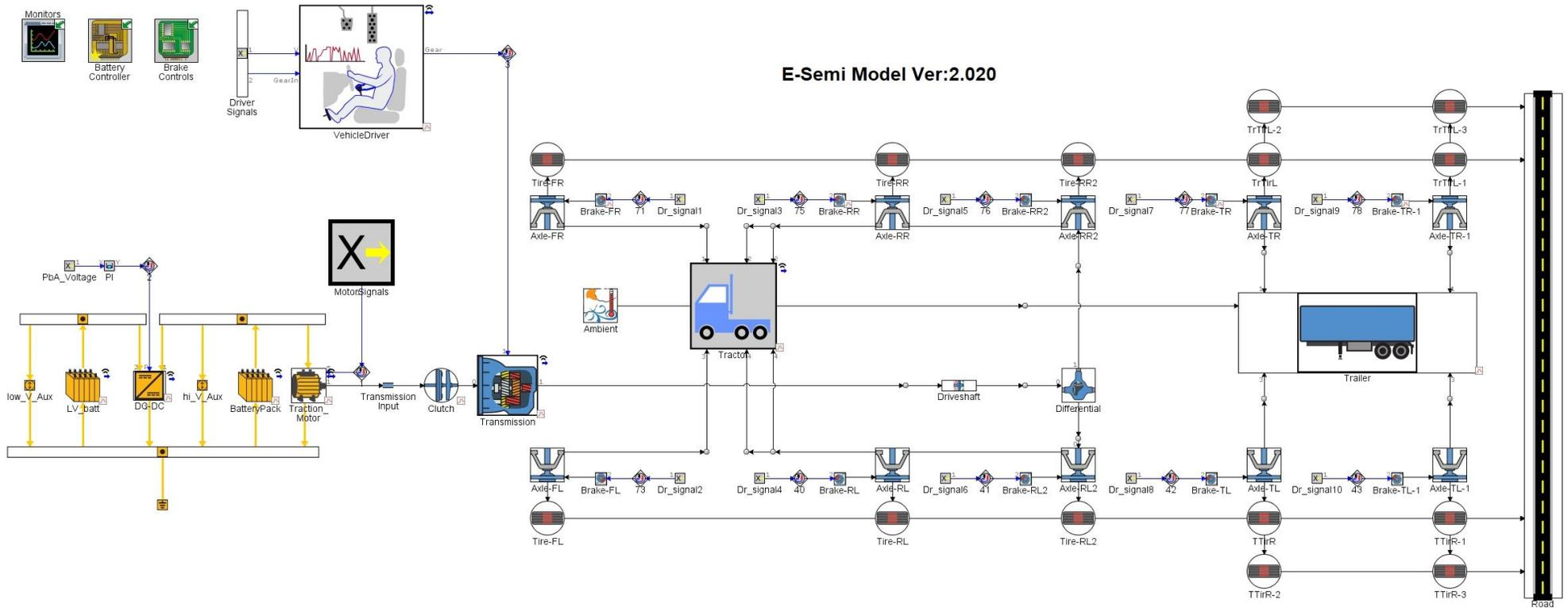
Figure 18: GT Suite model of the electric tractor-trailer
