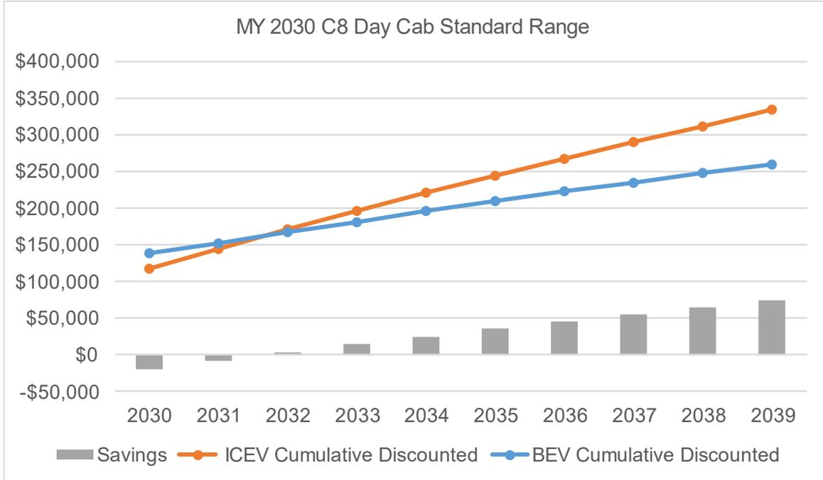
**Figure 52: TCO parity of an MY 2030 Class 8 day cab standard range with depot charging.**
