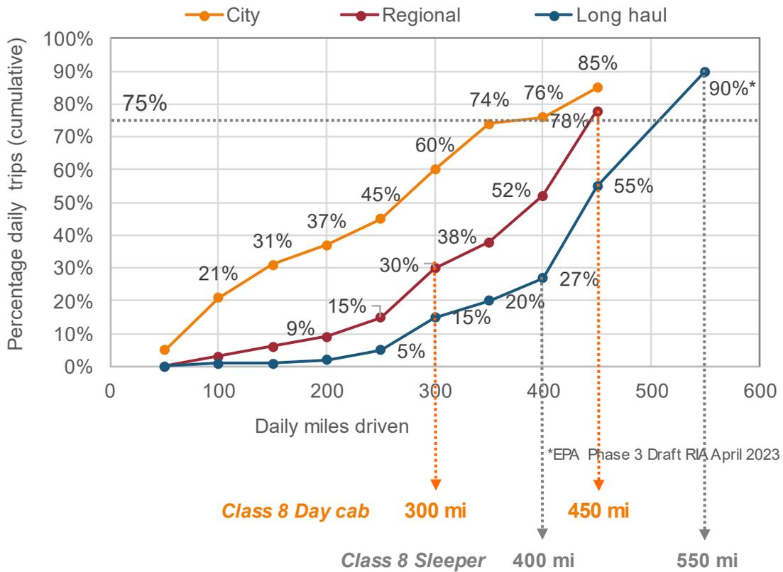
Figure 15: Typical Daily VMT by segment based on NACFE and ACT study of 2018. Cumulative percentage of tractor-trailers under a particular daily mile driven (calculated from Table 3).
