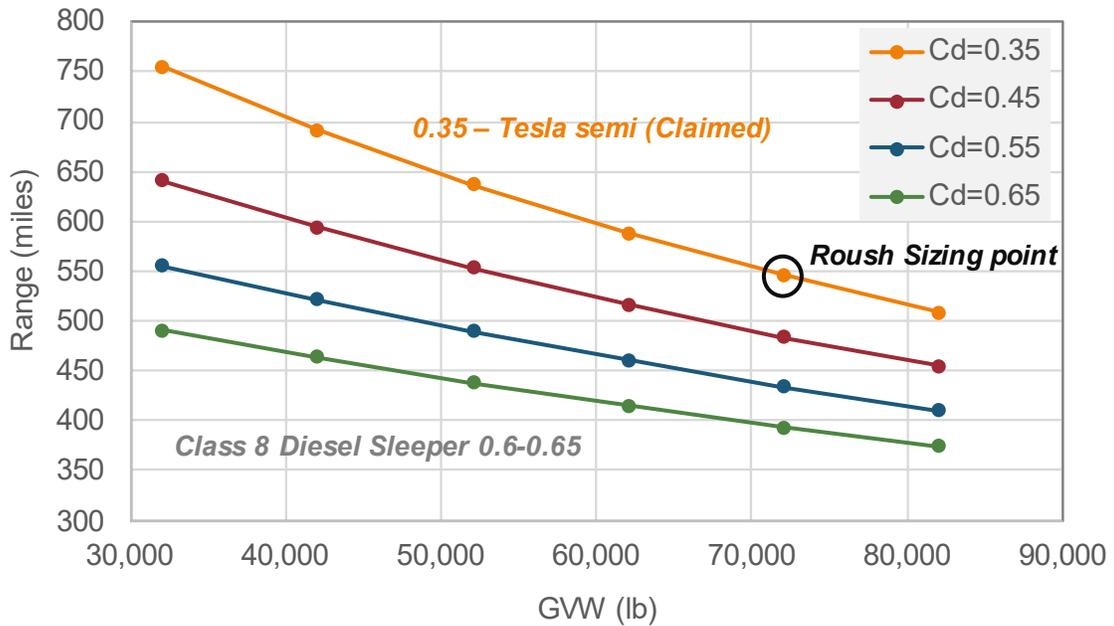
**Figure 21: Effect of coefficient of drag on energy efficiency**
