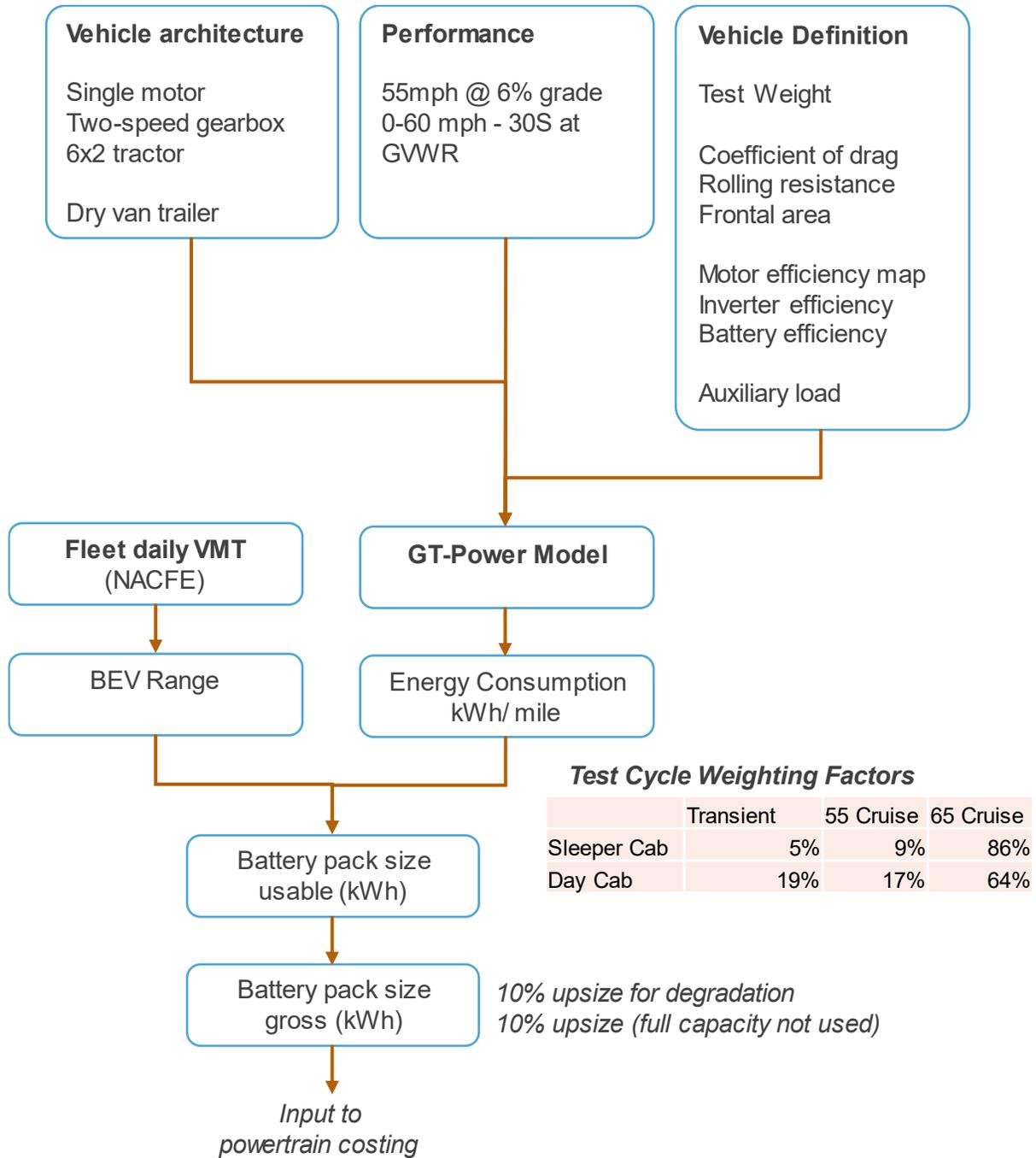
**Figure 13: Methodology for powertrain sizing (input to powertrain costing) and energy consumption (input for TCO calculation)**
