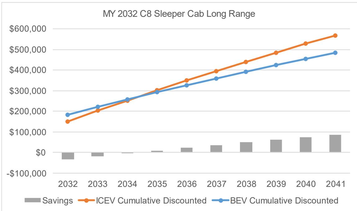
**Figure 59: TCO parity of an MY 2032 Class 8 sleeper cab long range with mixed charging scenario.**
