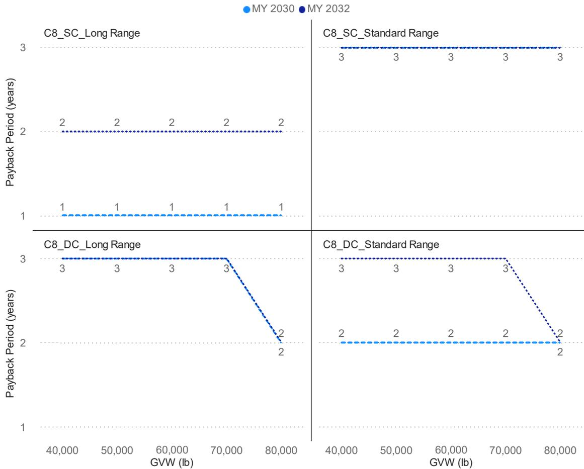
**Figure 6: Effect of GVW on the payback period**
