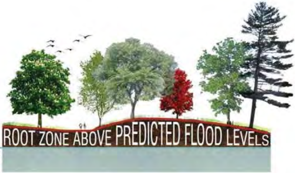
Raised grade level accounts for 2 feet of sea level rise by 2100, allowing for new tree roots to grow above future flood elevation.
