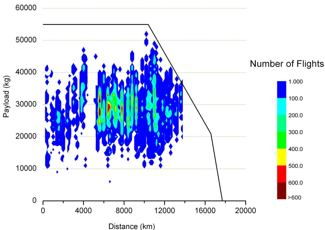
**Figure 1 Average operational norms for Boeing 777-200 aircraft as reported in BTS form 41 data (code 627). The black boundary line represents the payload-range capabilities for B777-200ER as quantified in Piano 5.**
