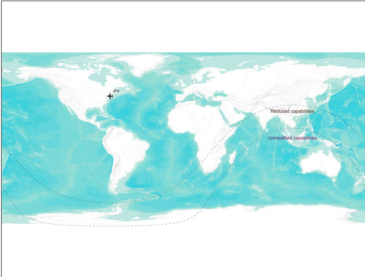
**Figure 2 Design range for the Boeing 787-8. Unmodified boundary as reported by Boeing. Reduced Capabilities is a 30% reduction in design range as modelled in Piano 5.**
