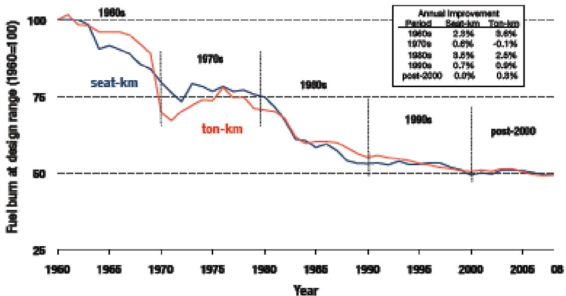
**FIGURE 1. AVERAGE FUEL BURN FOR NEW AIRCRAFT, 1960-2008**
