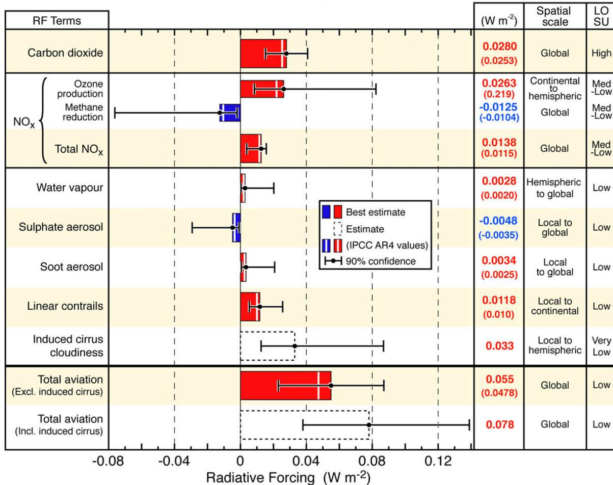
Excluding the effects of induced cirrus, the overall radiative forcing by aircraft is a factor of 1.9 times greater than the forcing by aircraft carbon dioxide emissions alone. However, to date, the focus of efforts in the EU and ICAO has been on CO<sub>2</sub>, justified by a lower level of scientific certainty surrounding the non-CO<sub>2</sub> effects and an ongoing debate on a suitable metric (although alternative, temperature-based metrics are already emerging).
