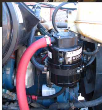
Figure 1 (above): Diesel particulate filter (Source: Clean Air Task Force)
