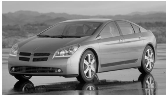
The Dodge ESX3 concept, unveiled by DaimlerChrysler in January 2000, showcased lightweight materials and a diesel-hybrid engine to achieve 72 MPG. (©2000 DaimlerChrysler)
