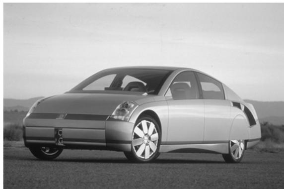
The GM Precept concept, unveiled in January 2000, was designed to achieve 80 MPG with a diesel-hybrid engine and the equivalent of 100 MPG with a hydrogen fuel cell engine. (©2004 General Motors and Wieck Media Services, Inc.)
