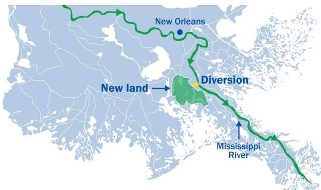
Louisiana’s land loss is largely due to a century of efforts to control the Mississippi River. The U.S. Army Corps of Engineers has built thousands of miles of dams, levees and other structures along the river to prevent flooding and ease navigation. These projects have also choked off the supply of sediment to the delta — sediment that raised south Louisiana out of the sea.
