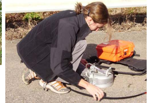
Flux accumulation chamber
