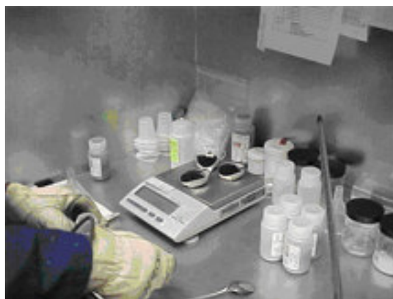
Figure 2. Ventilated Enclosure/Weigh-up with CNTs in pans (12/20/05)
