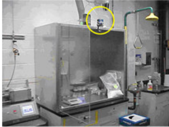
Figure 6. Ventilated Enclosure/Weigh-up with air sampling device (2/8/06)
