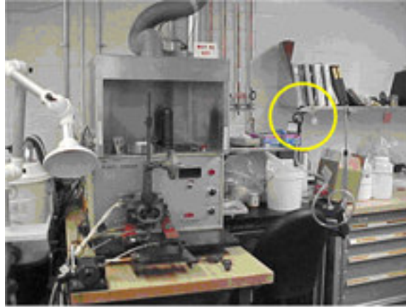
Figure 9. Brabender Plasti-corder Batch Mixer with air sampling device (2/8/06)
