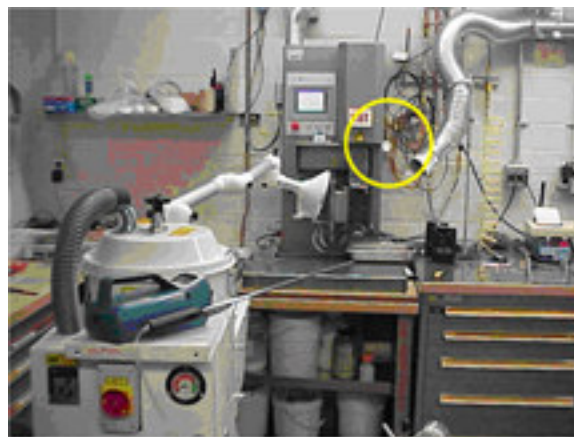
Figure 4. Batch melt with air sampling device and HEPA ventilation system in place for loading material (12/20/05)
