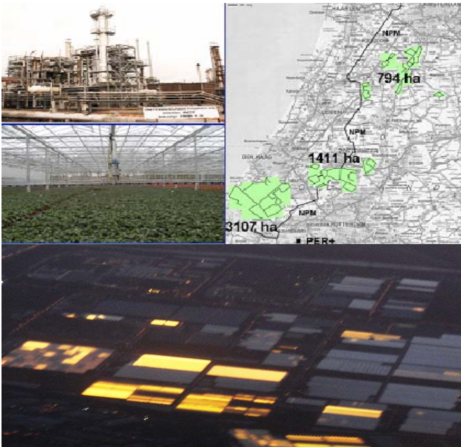
Capturing oil refinery CO 2 (at the map named 'PER+') and transferring via pipelines to Westland greenhouses. Clockwise, from upper left: Shell Pernis Refinery; map of pipelines; aerial view of greenhouses at dawn; interior view of greenhouse. Photo credits: Jos Cozijnsen
