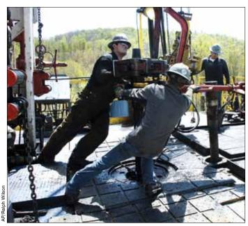
Natural gas well site in Pennsylvania. Hydrofracturing (fracking) blasts water, chemicals and sand into rock under very high pressure to release the shale gas.
